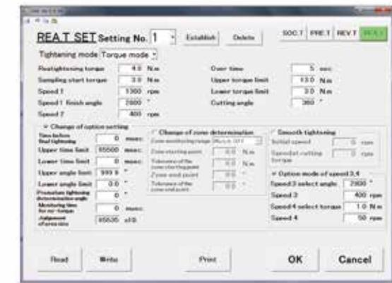
Screen for setting the final tightening. For the type of final tightening, two types; torque method and angle method are available
