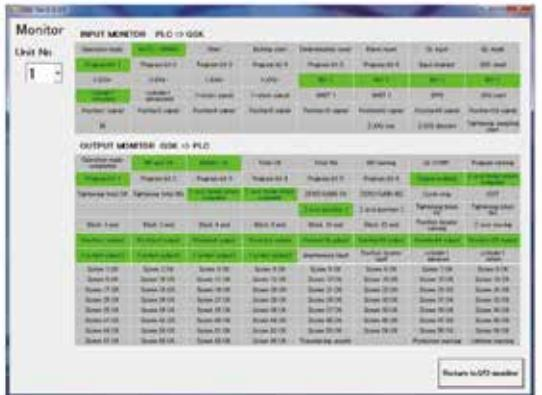
Screen for checking the I/O status with upper link.
