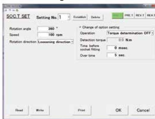
Screen for setting the rotation for matching a bolt with a socket
