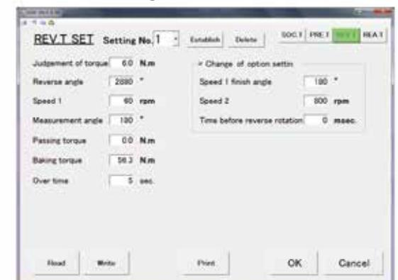
Screen for setting seizure judgment after temporary tightening of bolt.
