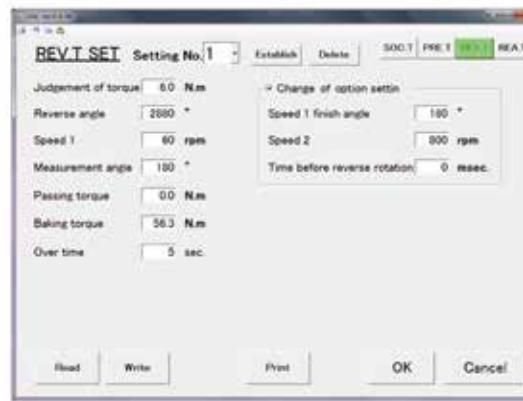
Screen for setting seizure judgment after temporary tightening of bolt
