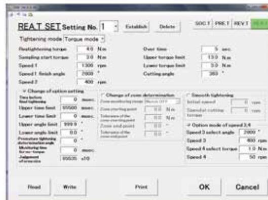
Screen for setting the final tightening. For the type of final tightening, two types; torque method and angle method are available.
