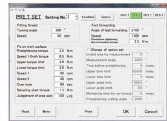
Screen for setting bolt setting status to seating (temporary tightening)
